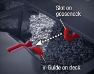
The V-Guide aligns the Slot on the gooseneck so you don't need to line up perfectly with the deck
